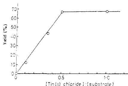
Figure 2. Yield (%) of chlorobenzene as a function of tin(II) chloride to substrate molar ratio. Reprinted with permission. Copyright 1981, The Royal Society of Chemistry.
